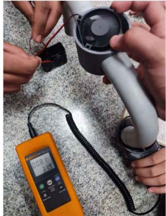
Fig. 6. Flow Measurement Using Anemometer
